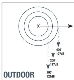
The following chart demonstrates the role distance plays in the "loudness" of an audible signal. Most of our devices are measured at a distance of 10 feet (on axis); Outdoor Warning Sirens are measured at 100 ft. (on axis). This gives us a common point for comparison.
